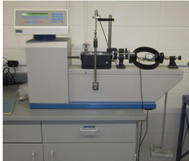
Figure 30. Drained direct shear test (ASTM D3080-04)
