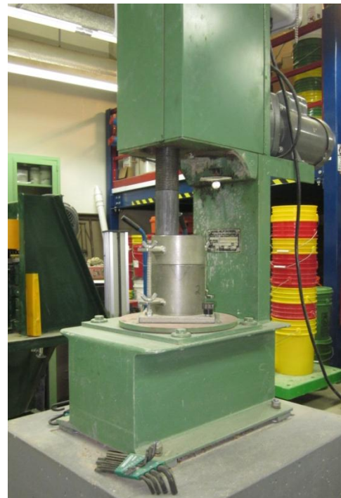
Figure 29. Standard Proctor test, method A (ASTM D698-00)
