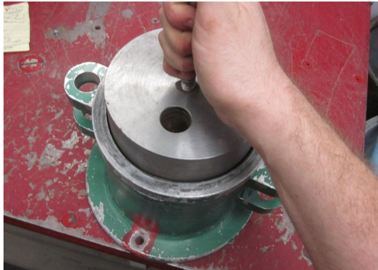
Figure 36. Surcharge plate extraction with removal rod
