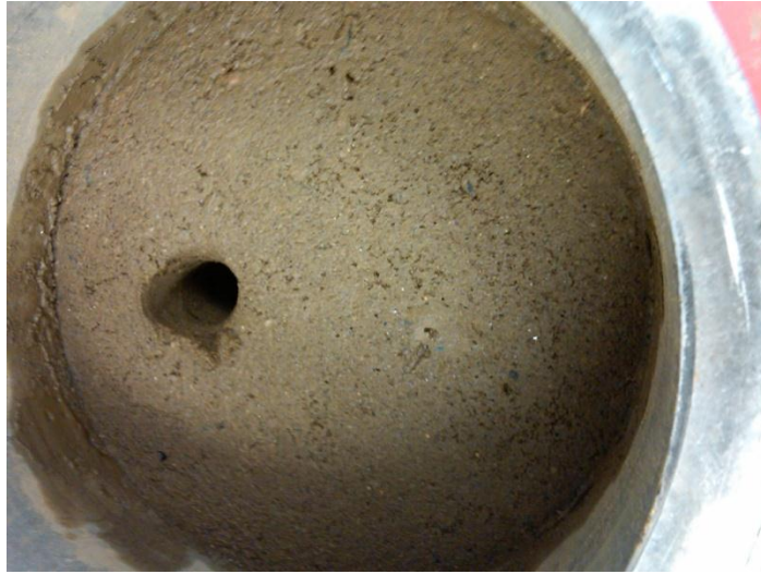
Figure 38. DCP borehole through sample in mold
