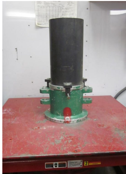
Figure 28. Relative density mold with surcharge on vibratory table (ASTM D4254-83)
