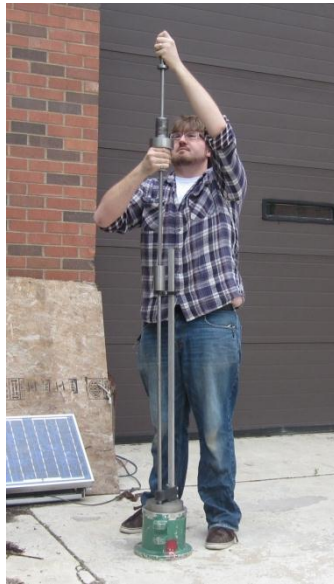
Figure 37. DCP test of sample in mold (4.6 kg hammer)
