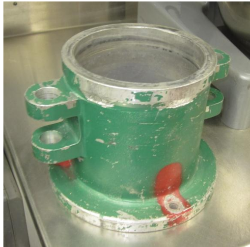
Figure 27. Relative density mold (ASTM D4253-83, D4254-83)
